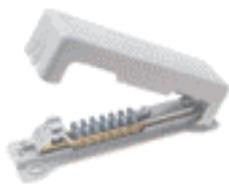
**small version**, for house systems up to 100A, nickel-plated brass, with plastic cover (sealable). With terminals for: 7 conductors of up to 25 mm<sup>2</sup>, 1 flat strip 30x4 mm, 1 round wire 8–10 mm
