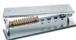
**large version**, with terminal bar 35x4 mm, hot-dip galvanised, base plate and cover made of sheet steel. With terminals for: 1 round wire 8–10 mm, 2 flat strips 40x4 mm, 1 copper cable of up to 50 mm<sup>2</sup>, 12 conductors up to 16 mm<sup>2</sup>
